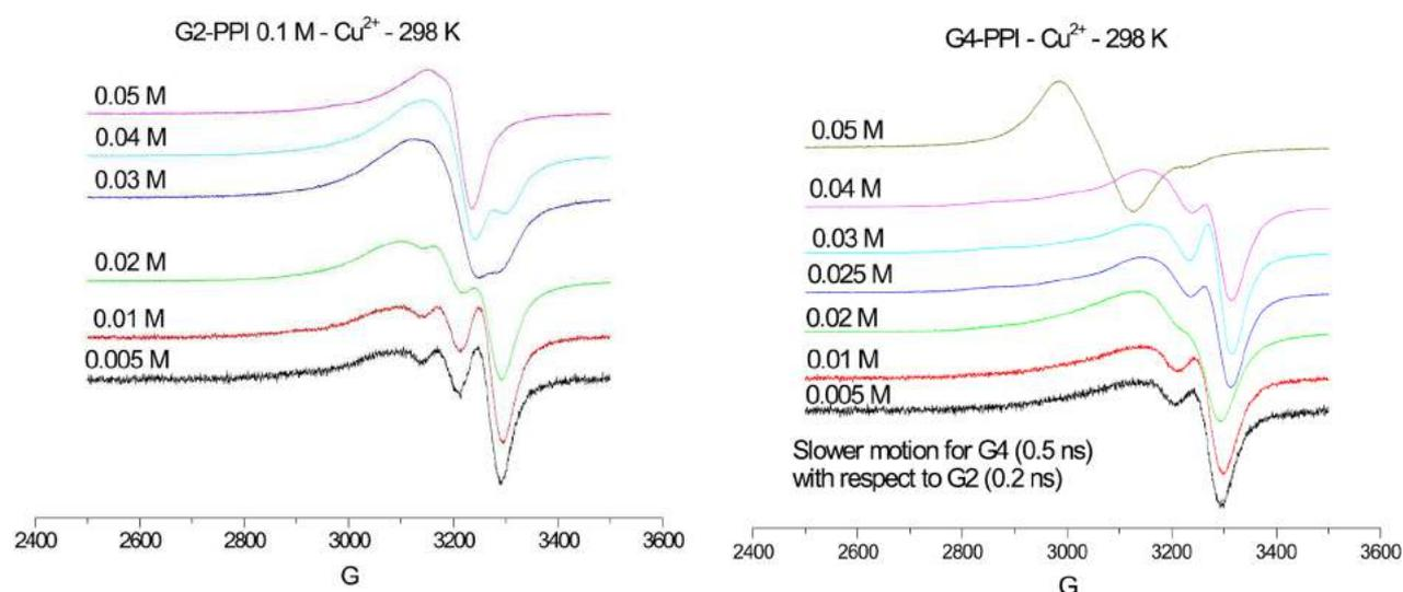
**Figure 7.** EPR experimental spectra ( $T = 298$  K) obtained for 0.1 M solutions of PPI-G2 (left panel) and PPI-G4 (right panel) at selected Cu (II) concentrations.
