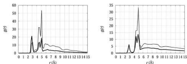
**Figure 5.** Radial distribution function ( $g(r)$ ) for N–N pairs in PPI-G2 (left, thick curve), PPI-G2 decorated (left, thin curve), PPI-G4 (right, thick curve), and PPI-G4 decorated (right, thin curve).
