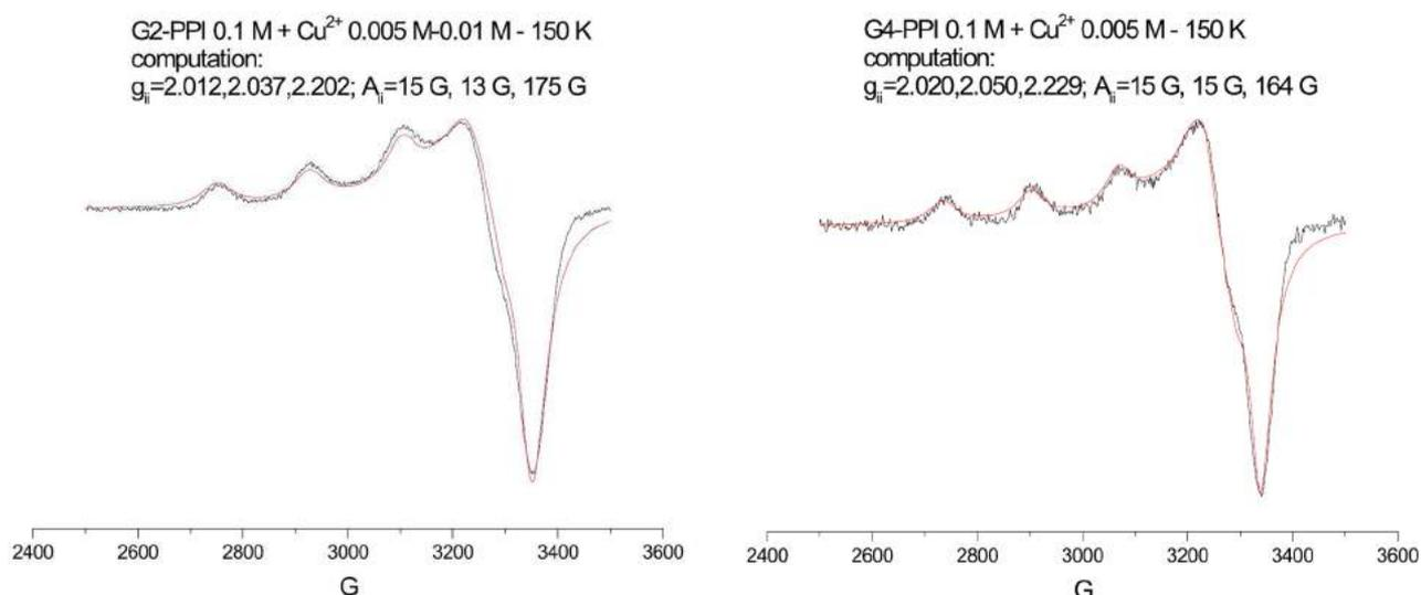
**Figure 8.** Experimental and computed EPR spectra of PPI-G2 (left panel) and PPI-G4 (right panel) at  $T = 150$  K and Cu(II) concentration of 0.005 M (for PPI-G2, the spectrum is almost invariant up to 0.01 M, while, at this Cu(II) concentration, the spectrum of PPI-G4 becomes similar to that of PPI-G2). The main computation parameters are reported in the figures.
