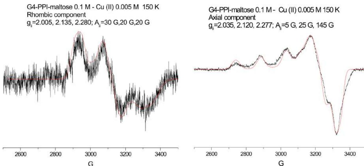
**Figure 10.** Computation of the rhombic (left panel) and axial (right panel) components of the spectrum of PPI-G4-mal (0.1 M) with Cu(II) concentration of 0.005 M (similar spectrum at 0.0025 M). The main parameters of computation are shown in the figure.
